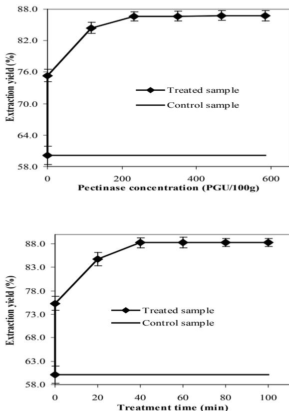
**Figure 3.** Effect of pectinase concentration (A) and treatment time (B) on extraction yield of pectolytic treatment of sonicated barbados cherry mash.
